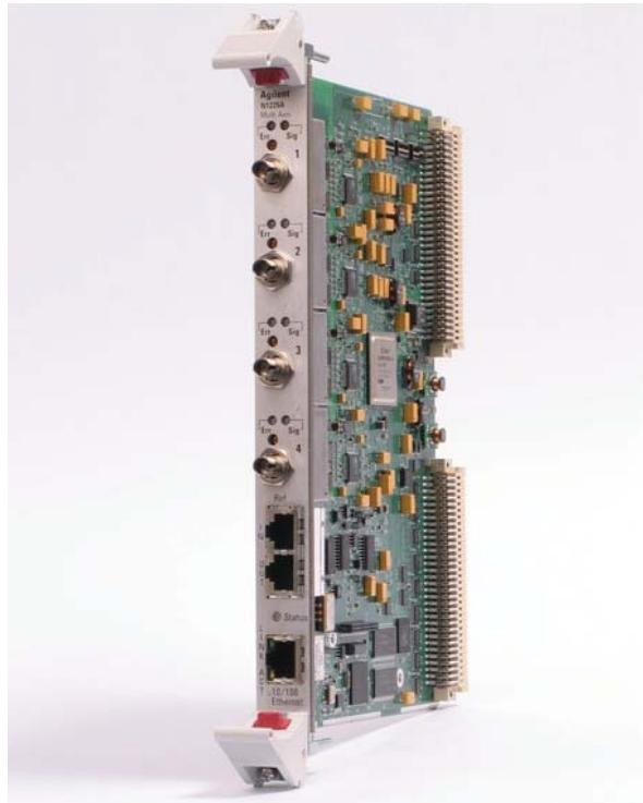
The N1225A axis board is a VME64x "6U" size board that supports a three-axis laser measuring system. The N1225A features a 0.15 nm plane mirror resolution, a ±10 m range, and a velocity limit of ±2.29 m/s when used with a 15 MHz split frequency laser head. The board requires a single +5V power supply and includes four high sensitivity receivers. To accommodate a greater number of axes, a digital reference can be passed between boards using Agilent-supplied Reference Passing patch cables.
